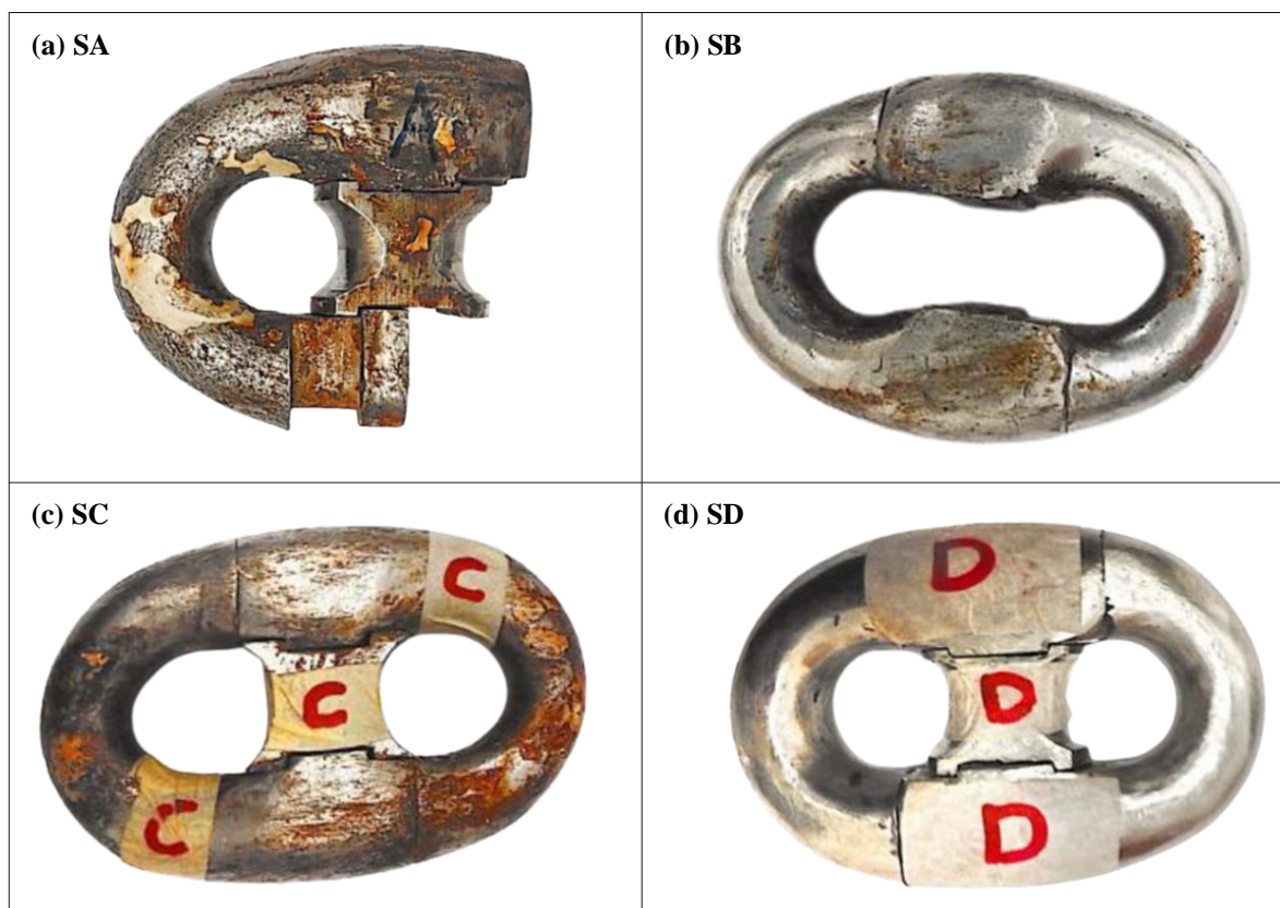
Figure 2: Tested LJS samples: (a) and (b) Broken LJS samples that failed during operation, labelled as SA and SB respectively. (c) Utilised LJS sample without any damage during operation, labelled as SC. (d) As-received LJS sample, labelled as SD.
